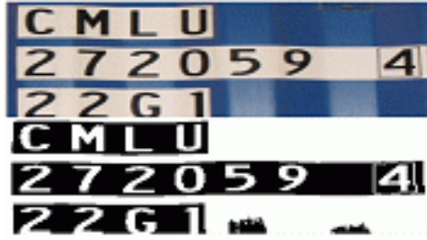
Fig. 6. Identifier area with white color and failed results of edge extraction
