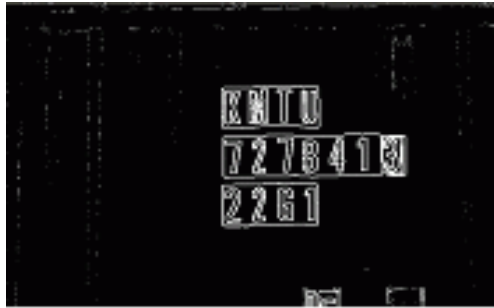
Fig. 4. Result of edge detection by fuzzy-based noise-removal and Sobel masking
