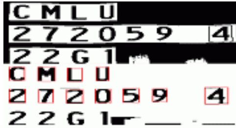
Fig. 7. Reversed binarized area of Fig. 6 and successful result of edge detection
