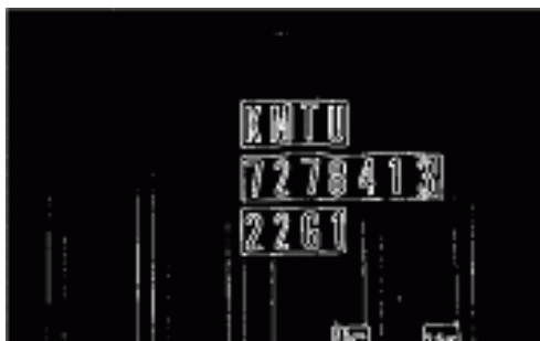
Fig. 3. Result of edge detection by only Sobel masking
